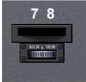
Finally we adjust the aileron trim. The aileron trim wheel is also mounted horizontally and since we're holding pressure to the right, we need to adjust the trim to the right until the airplane doesn't "roll off" towards the heavy left wing.
